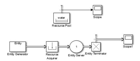
**6** Simulate the model and observe the amount of resources in use (Scope).
