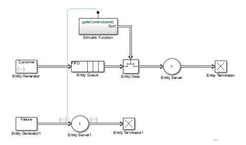
**Note:** A gate prevents new entities from arriving at the server but does not prevent the current entity from completing its service. If you want to eject the current entity from the server upon a failure occurrence, then you can use the preemption feature of the server to replace the current entity with a high-priority "placeholder" entity.
